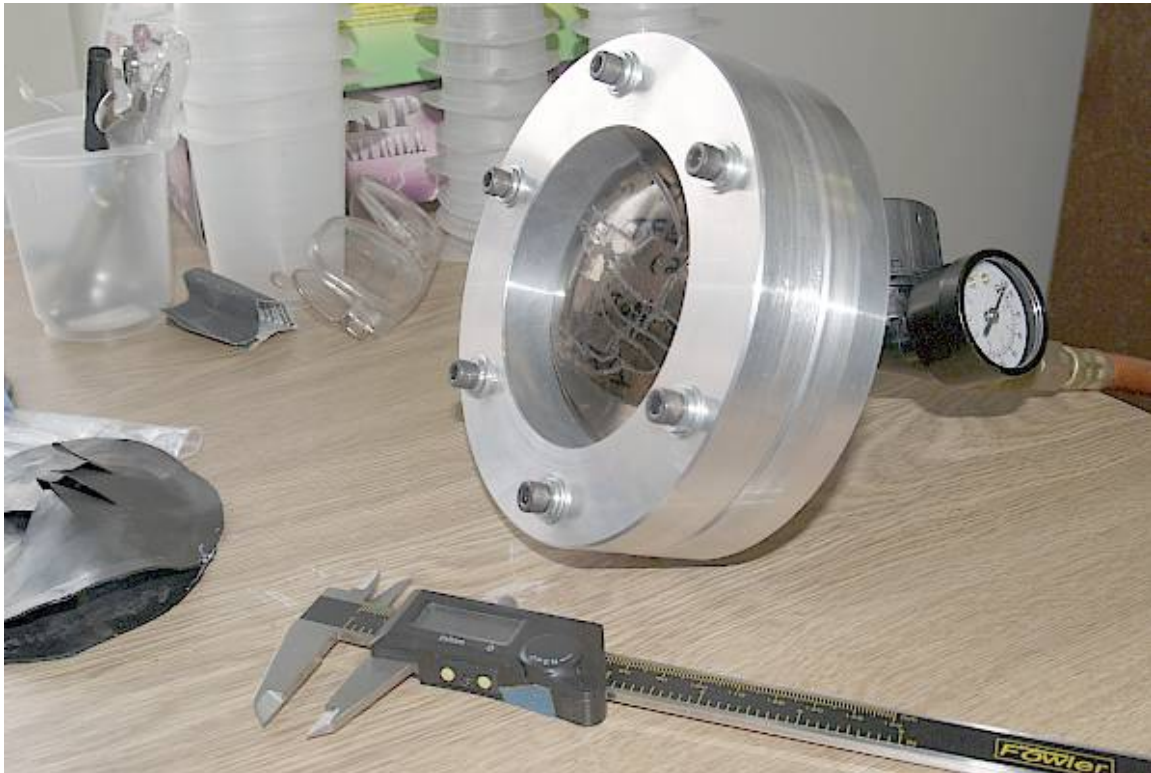
Figure 1: The “Puffer” used to Apply Biaxial Strain to Laminated Rubber Samples
